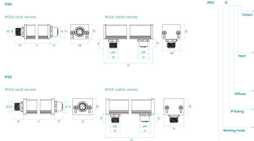
YL - M12A radial female connector PY - 10 cm axial cable with M12A female connector **RY** - 10 cm radial cable with M12A female connector Κ - Axial Cable, 2 m KL - Radial Cable, 2 m - M12A axial male connector YL - M12A radial male connector PY - 10 cm axial cable with M12A male connector RY - 10 cm radial cable with M12A male connector - Semidiffuse С U - Ultradiffuse - IP40 3 - IP65 5 P - Power Е - Eco D - Dual: Power/Eco ▶ 1 - 18 - 75 mm steps Length
