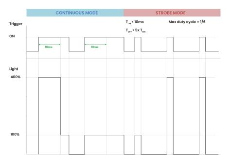
For Strobe mode operation, it is recommended that the power supply be twice as powerful as the Strobe mode lamp.
